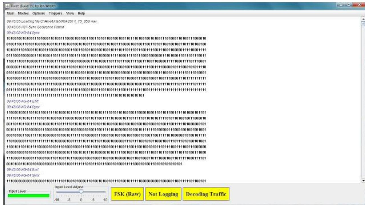
Both types of triggers can be seen (in blue text) when activated and the KG-84 messages (or blocks of a message) are clearly defined.
