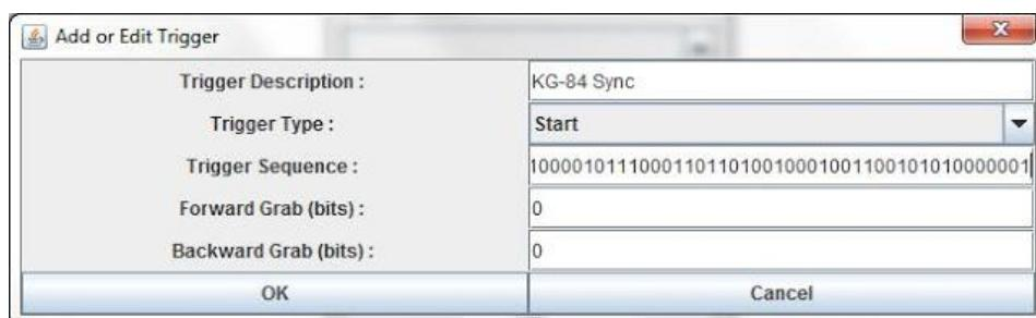
(you can cut and paste the binary value from this blog post rather than typing it in yourself). After that click on the OK button in this dialog box followed by the OK button in the Modify Triggers dialog box. Once you have done that the program will return to the main screen and automatically save the trigger to your hard disk.
