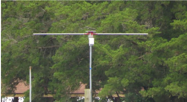
One of the Wallops VIPIR receive antennas
